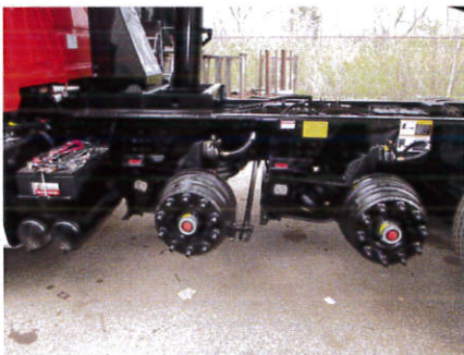
Auxiliary air lift axles allow for increased GVWR and maximum payload.
