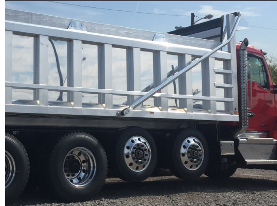
Auxiliary air lift axles allow for increased GVWR and maximum payload.
